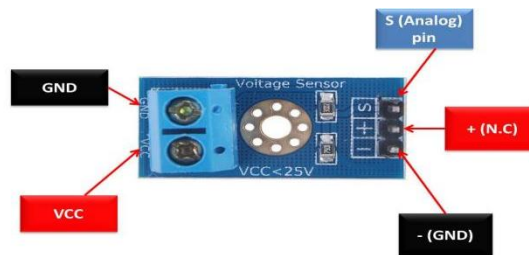
Fig 6.Voltage Sensor Pin Configuration
