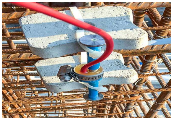
Fig 3:Concrete-embedded vibrating-wire strain gauge (GEOKON Model 4200) bonded to rebar in a bridge deck
