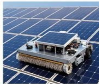
Robotic Solar Cleaner in Action
