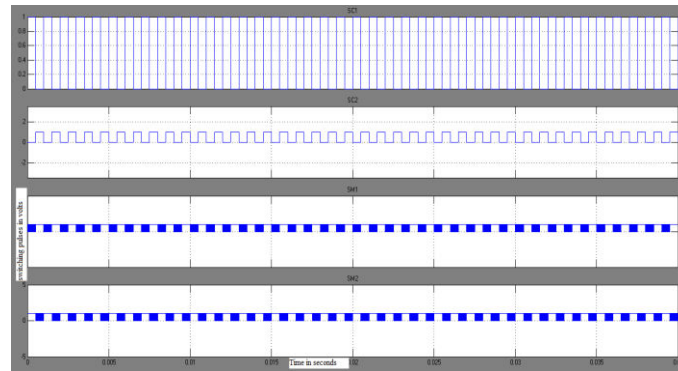
Fig.7..Switching pulse waveforms for three stage
